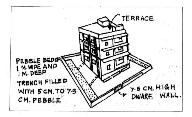
On the three sides along the inner periphery adjoining the compound wall, dig 1m. wide pit to a depth of 1.5 m. and fill it with 5 to 7.5 cm. sized pebbles let the rain water falling on the terrace flow into this pebble bed.
