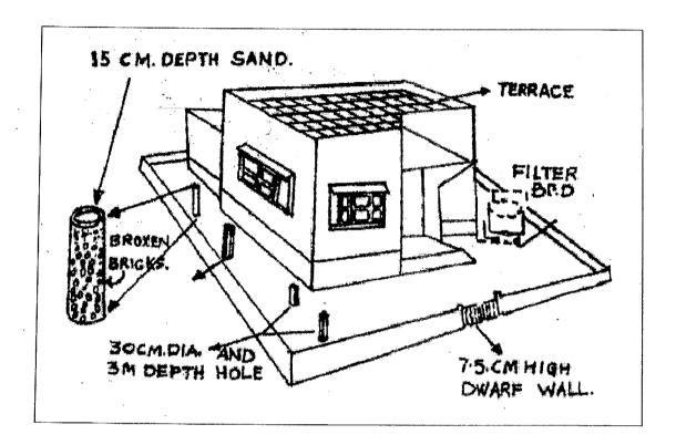
Dig a number of 3 mtr. deep and 30 cm dia percolation pits at an interval of 3 mtrs. around the plinth fill them up with broken bricks and pack the top 15 cm. with river sand. Erect 7.5 c.m. high dwarf walls entrance to facilitate recharge.
